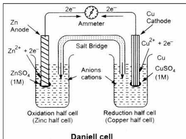
The two half-cells of a voltaic cell are connected by a salt bridge. A salt bridge is a tube of an electrolyte in a gel that is connected to the two half-cells of a voltaic cell; the salt bridge allows the flow of ions but prevents the mixing of the different solutions that would allow direct reaction of the cell reactants. The half-cells are connected externally so that an electric current flows.
