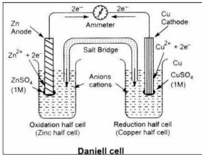
The two half-cells of a voltaic cell are connected by a salt bridge. A salt bridge is a tube of an electrolyte in a gel that is connected to the two half-cells of a voltaic cell; the salt bridge allows the flow of ions but prevents the mixing of the different solutions that would allow direct reaction of the cell reactants. The half-cells are connected externally so that an electric current flows.
