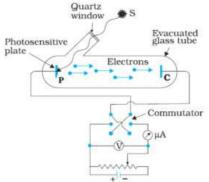
Fig.: Experimental arrangement for study of photoelectric effect.
