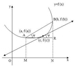
There exists a point  $(c_1 f(c))$  on the curve such that the tangent there at is parallel to the chord joining the end points of the curve.
