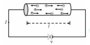
The electron current  $(I_e)$  and the hole current  $(I_h)$  constitute the current I flowing through the semiconductor i.e.
