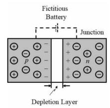
The thickness of the depletion layer is of the order of  $10^{-6}$  m.
