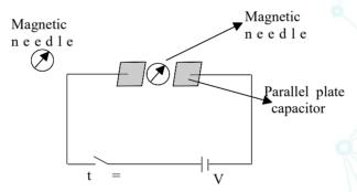
Deflection of needle (1) is under stood as M.F. is produced due to current flowing in the wire.
