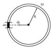
Here we can simply state that another element of same mass exactly opposite to dm on other half of ring will produce an equal gravitational field at C in opposite direction. Thus due to all the elements on ring, the net gravitational field at centre C will be vectorially nullified and hence net gravitational field strength at C will be 0.
