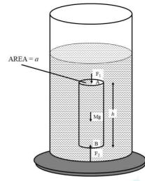
In order to calculate the pressure difference between points A and B, consider an imaginary cylinder of liquid of cross-sectional area *a*, such that points A and B lie on its upper and lower circular faces respectively. Obviously, the length of the cylinder will be h and it will contain liquid, whose weight is given by
