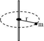
In translation motion, the mass of a body m given measure of the inertia of a body. But in rotational motion moment of inertia depends on mass of body as well as on its distribution about the axis of rotation.
