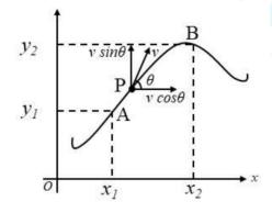
If along the curve particle moves a distance dr in time dt, we define v=dr/dt. Similarly, when particle moves dr along the curve, its x-coordinate changes by dx and y-coordinate changes by dy. Thus the velocity projections can be written as
