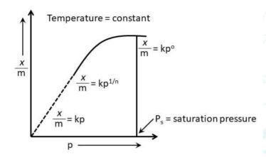
(a) At very low pressure: At very low pressures, the graph is nearly straight line.
