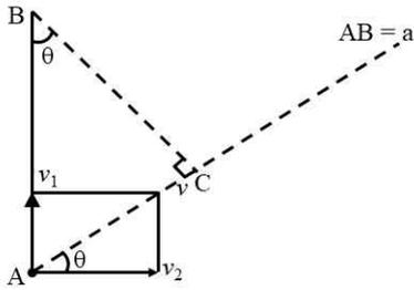
$$\sin\theta = \frac{V_1}{\sqrt{V_1^2 + V_2^2}} = \frac{V_1}{V}$$
