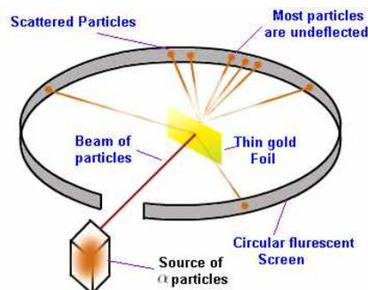
H. Geiger and E. Marsden performed an experiment on  $\alpha$ -particles scattering, in 1911, as suggested by Ernst Rutherford.
