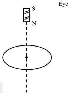
**Solution 1** As per Lenz's law, induced current in the loop will be such that it will oppose the cause of change in flux (that is motion of the bar magnet towards itself). Thus current flows in the loop so that it is equivalent to a bar magnet with its North facing the approaching North pole of the magnet thereby repelling it. Thus current for the observer will be anticlockwise.
