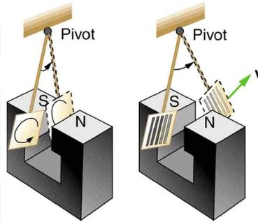
Fig. Eddy currents are generated in the copper plate, while entering and leaving the region of magnetic field.
