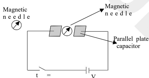
Deflection of needle (1) is understood as M.F. is produced due to current flowing in the wire.
