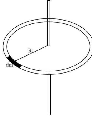
Above figure shows a ring of mass  $M$  and radius  $R$ . To find its moment of inertia, we consider an elemental mass  $dm$  on it (see figure). When the ring rotates, the element  $dm$  will revolve in a circle of radius  $R$ , infact here radius of all the elements taken on ring will be same  $R$ .
