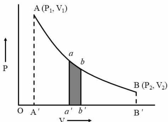
Let  $a$  be any point on the indicator diagram and  $P$  and  $V$  be the values of pressure and volume corresponding to it. Suppose that volume increases to  $V + dV$  corresponding to point  $b$  on the indicator diagram, such that the pressure remains constant.
