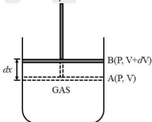
If  $a$  is are of cross-section of the piston, then force on the piston will be equal to  $P a$ . Therefore,
