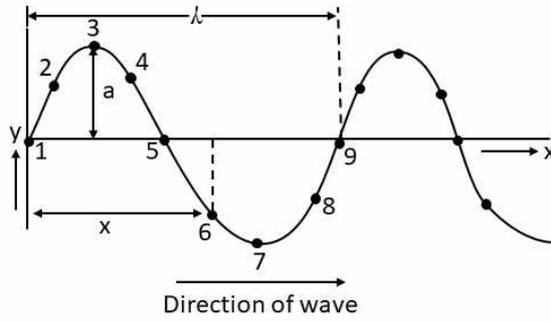
$$y = a \sin \omega \left( t - \frac{x}{v} \right) \quad \text{But } \omega = 2\pi n, \quad y = a \sin (\omega t - kx) \left( k = \frac{\omega}{v} \right) \dots \text{(i)}$$
